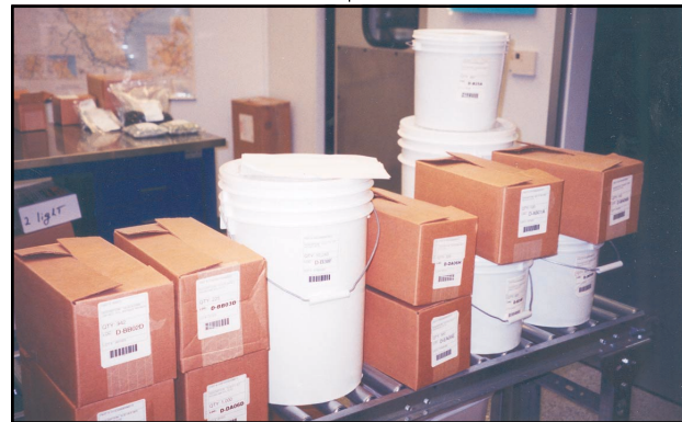
All products received are re-packaged into one of four container sizes. They are labeled with all needed identifying information including the unique bar code. Each package is "random stocked" into the next available location for that size package.
