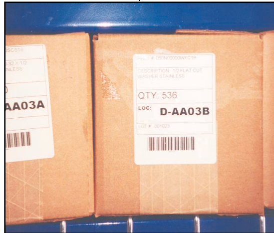
Each label has a single bar code that identifies all aspects of the package, including Part Number, Quantity, Weight, Lot Number and Inventory Location. The system also prints a Receipt Label to be attached to the Receiver to confirm the arrival of the goods.
