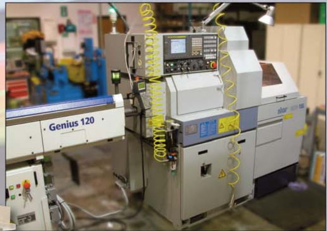
Star SB16 16MM CNC Swiss Lathe for Small Measuring Tool Probes
