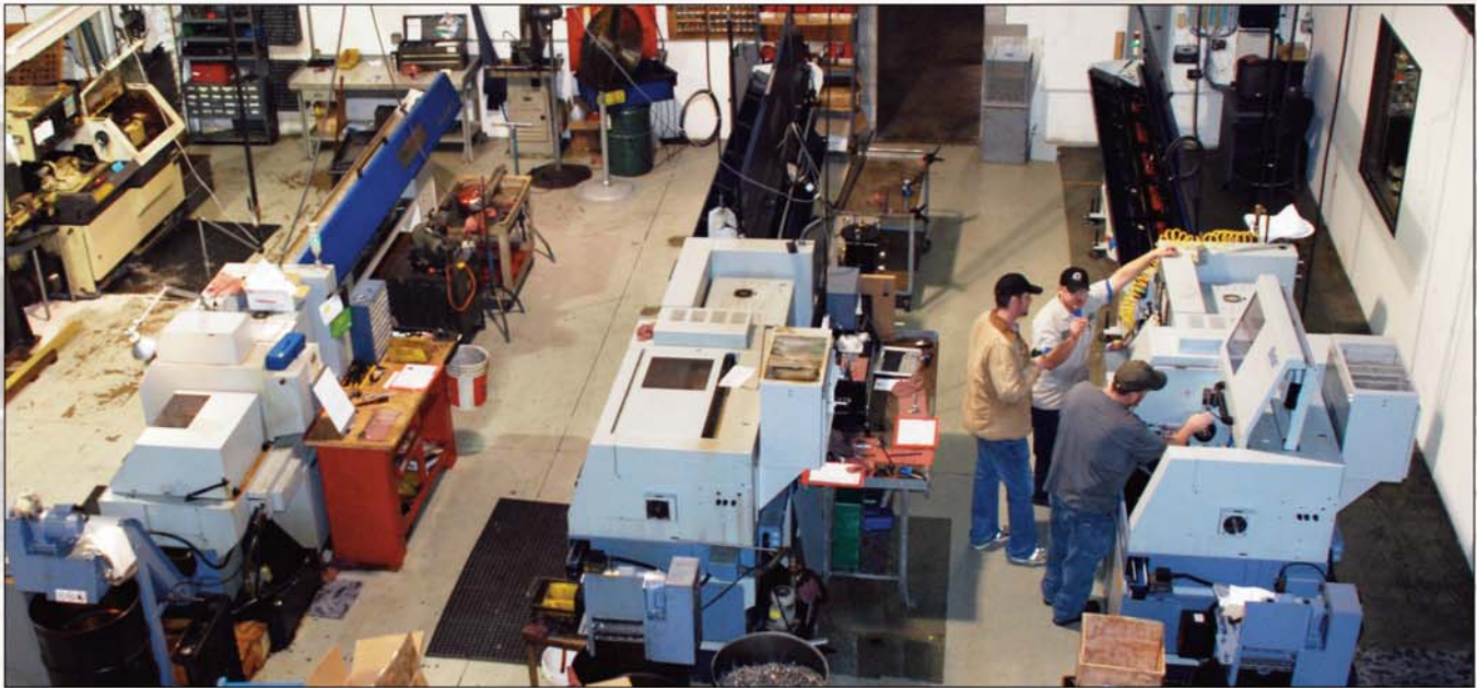
Partial View of CNC Swiss Lathe Area – (3) Star CNC Swiss Lathes with Bar Feeds – 1.250" Capacity
