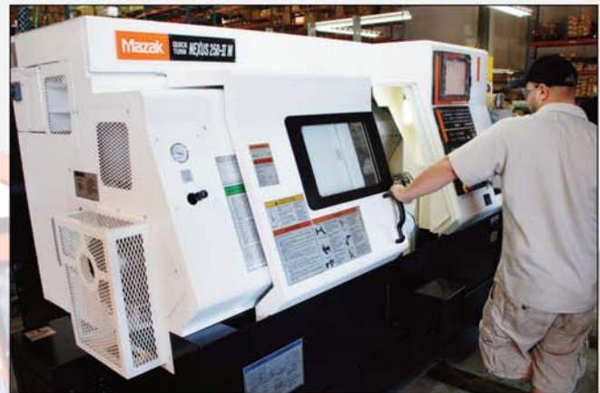
Mazak Nexus Quick Turn CNC Lathe – 3" Thru the Spindle Capacity, and 14.75 Diameter X 19.85 Length Chucking Capacity
