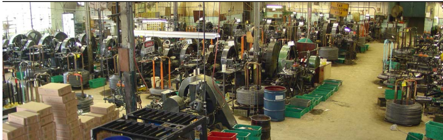
Manufacturing floor (42 machines heading 3 million rivets per day)
